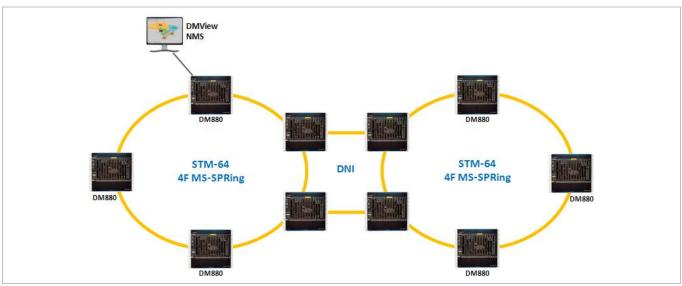
STM-64 4-Fiber MS-SPRing Dual Node Ring Interworking (DNI)
