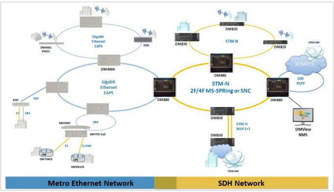
SDH Transport and Aggregation, with Seamless Metro Ethernet Network Integration
