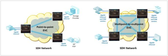
Point-to-Point and Multipoint-to-Multipoint Ethernet Virtual Connection (EVC) over SDH Network
