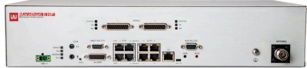
Marathon II unit with 4 x 10/100/GE Ethernet, 4 x balanced E1 and 2 x V.24/V.28 Serial ports
