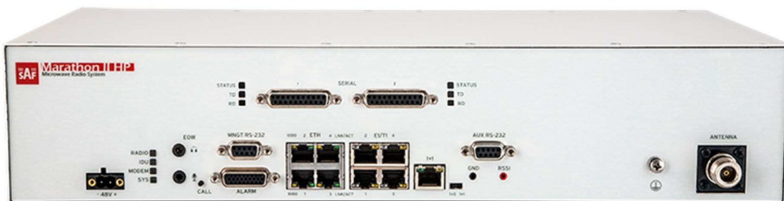
Marathon II HP with 2x DB-25 V.24/V.28 Serial interface ports
