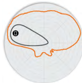
Figure 5. T750 5GHz Elevation Antenna Patterns
